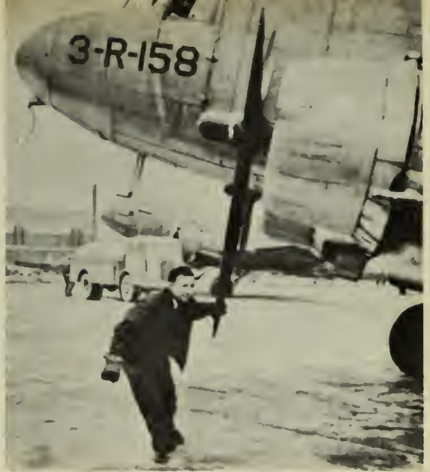
SOP IN '43 was pulling oil from behind plane's pistons.
